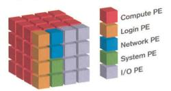
Jobs are submitted interactively from login PEs using the Cray XT3 job launch command, or through the PBS Pro™ batch program, which is tightly integrated with the system PE scheduler. Jobs are scheduled on dedicated sets of compute PEs and the system administrator can define batch and interactive partitions. The system provides accounting for parallel jobs as single entities with aggregated resource usage.
