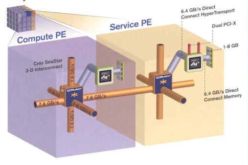
Cray XT3 System Sample Configurations
