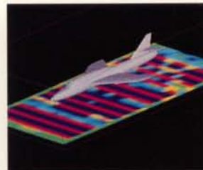
Electric field intensity around a military aircraft. The figure shows the variation (red is negative and blue is positive) of the vertical component of the electric field throughout a plane close to a military aircraft. Results obtained by EMMA T2 code. PATRAN has been used for preprocessing and visualization is via AVS.
