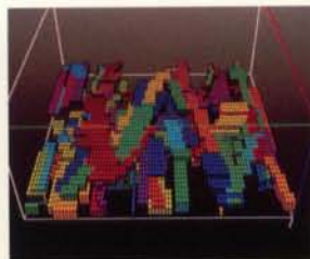
Petroleum reservoir simulation used for recovery profile predictions. Each color represents a particular grouping of sand bodies. Simulations performed with the three-dimensional, compositional simulator VIP-EXECUTIVE.
