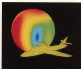
Radar cross section (RCS) of a military aircraft. Red indicates regions of high RCS and blue indicates low RCS. Calculations performed using a frequency domain code with an out-of-core solver from the EMMA software suite. PATRAN has been used for preprocessing and visualization is via MPGS.
