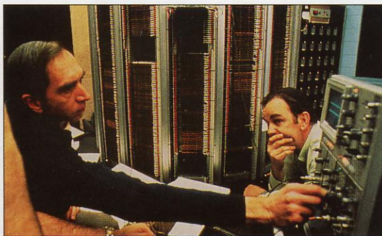
Davis in 1979 with the CRAY-1: Cray's engineering team devised a Freon-based cooling system that mimimized the machine's searing heat inside the processor.
