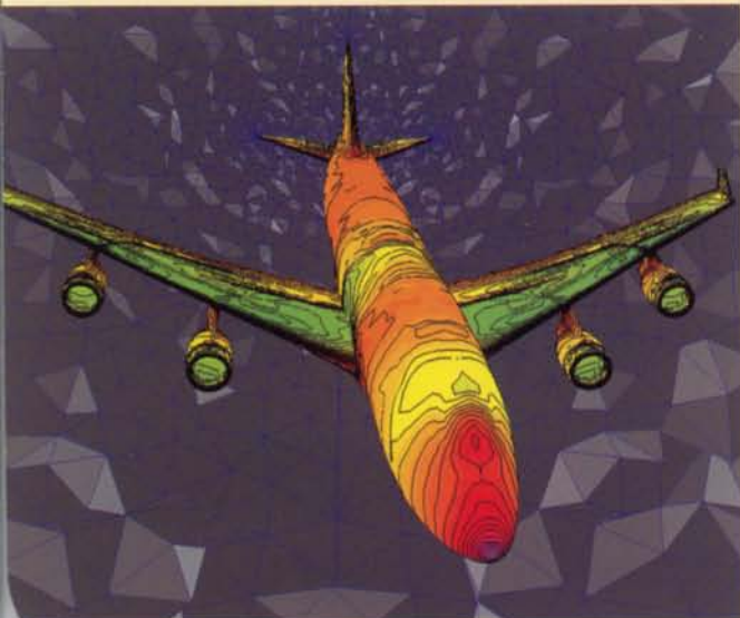
Computational fluid dynamics simulation of an aircraft in flight.
