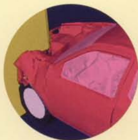
Simulation of an offset barrier frontal collision.
