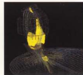
Right, flame front and velocity field at auto-ignition in a Nissan Motor Company indirect injection diesel engine, generated by CRI/TurboKiva.
