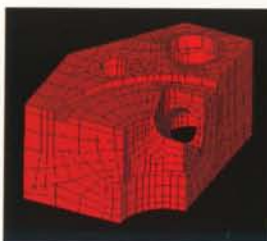
Left, cylinder head model with 192,000 degrees of freedom and 2400 RMS wavefront, analyzed with the ABAQUS software package.
