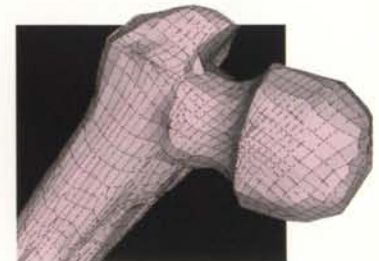
Right, mesh of a human femur model containing 14,887 elements, used for analysis with the ABAQUS analysis program, and generated with the Hexar mesh-generation software.
