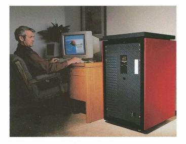
The CRAY EL92 deskside computer system delivers CRAY Y-MP and CRAY C90 compatibility to an office environment at a low price point. With up to two processors and 512 Mbytes (64 Mwords) of central memory, the CRAY EL92 system offers a clear upgrade path to large-scale parallel Cray Research supercomputing.
