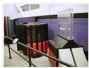
A Cray-2 and its Fluorinert-cooling "waterfall", formerly serial number 2101, the only 8-processor system ever made, for NERSC
